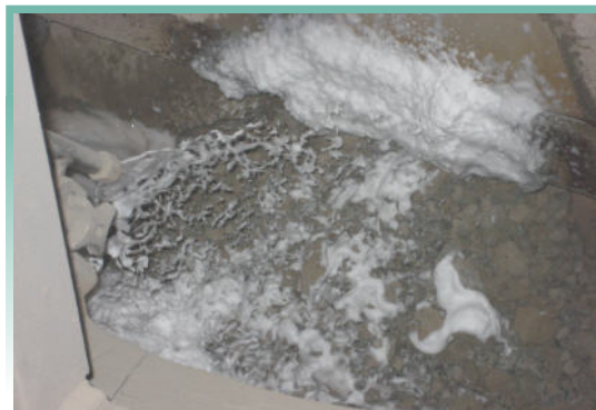
Foam spray added to limestone at a crusher inlet
