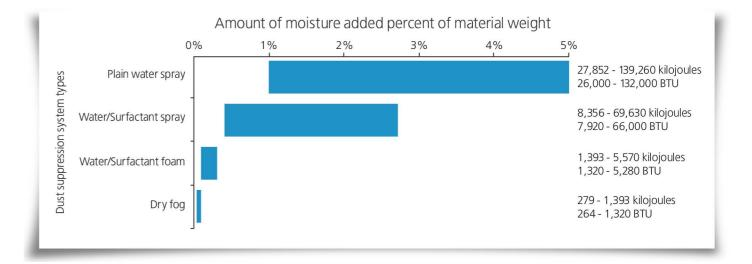
Because a "plain" water spray requires the highest volume of moisture for effective dust suppression, this method extracts the highest thermal penalty. While the use of a simple water spray for dust suppression may be a lower cost because the water is readily available and there is less "out-of-pocket" expense, the penalty for the addition of surplus moisture can be very costly indeed.
