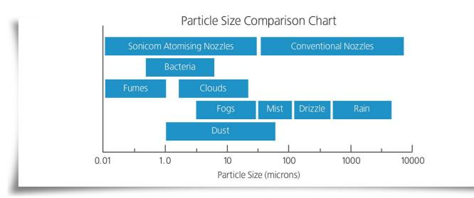
The "dry fog" dust suppression system controls respirable particulates down to the 0.1 to 3 microns which are considered to be the principal source of dust clouds, haze and accompanying low levels of visibility. In most applications where respirable dust particles can be settled out of the atmosphere quickly, the sonicom system makes it unnecessary to add a tension additive product to the water.
