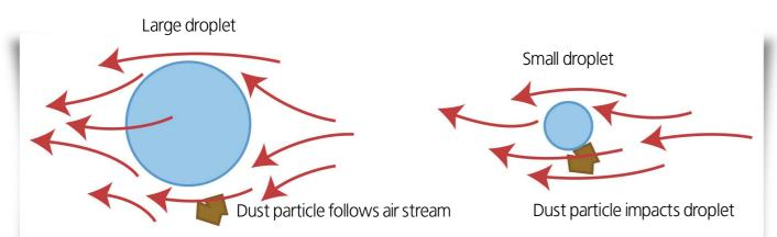
Diagram illustrates the importance of droplet size for particle agglomeration. Airflow around the large water droplet (left) prevents the dust from contacting the droplet. However, the dust particle easily impacts the small droplet (right) triggering agglomeration.
