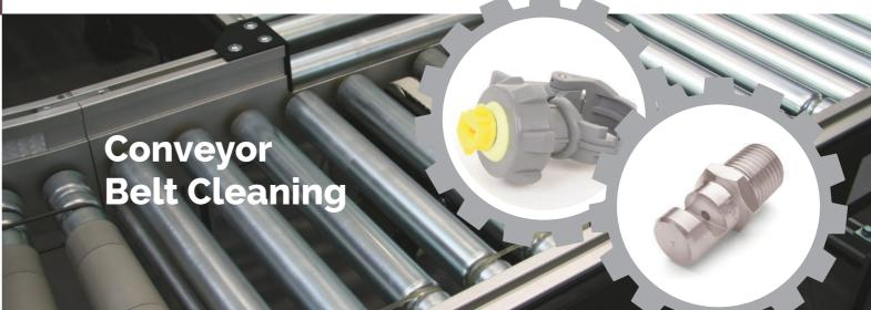
Conveyor belts carrying food products require regular cleaning to ensure that hygiene standards are maintained. Cleaning efficiency can be improved significantly by using fixed spray nozzles in place of manual operator based cleaning.
